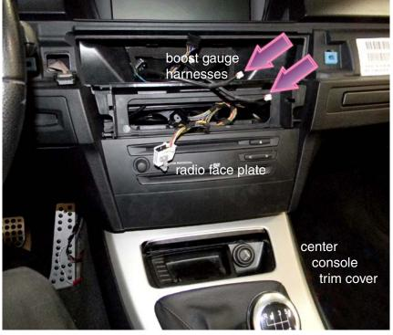
Before you start reassembling the dash make sure you have routed the gauge power harness and transducer harness to the vent opening in the dashboard (arrows).
