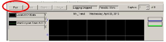
14. Press the *DI1* pushbutton then push the *DI0* and watch the trend capture the data of the Timer.ACC.
