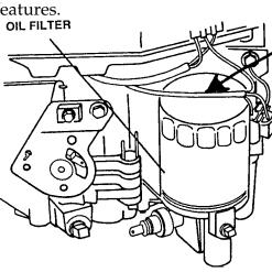
POKE HOLE IN TOP OF FILTER HERE.
