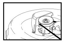
Always mow grass with all safety guards required installed on the mower deck.
