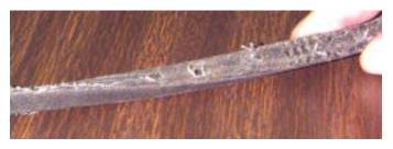
**V-belt Abrasion from idler locked up** The vbelt will be worn across the width of the belt. The material will be carbonized and show cracks.
