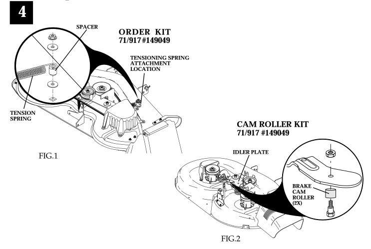
FIG. 1 - Tensioning spring on electric clutch 44"/50" decks break - Solution - order kit 71/917 #149049
