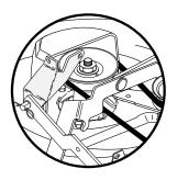
42" mower deck 1992 TO 1993 OLD STYLE ARCH SUSPENSION TEE PATH BELT ROUTE WITH TWO IDLER PULLEY. USE DECK BELT 71/917 #130969 SIZE 1/2 X 11/32 X 92.41
