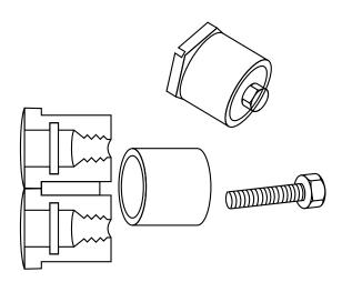
The drive components on the current inertia drive starters are held in position by a snap ring that fits in a groove near the end of the armature shaft. Because the ring is partially recessed in the groove, removal and reinstallation can be tricky and even hazardous. Our "Tool of the Year" is a small kit that will do the job quickly, easily, and safely.
