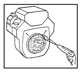
4. The marks you made on the blower housing, corresponding to the firing points of the cylinders, should be 90° apart. As you accelerated, the timing should have advanced 5 to 15, and the line on the screen should have moved 1/2" to 3/4" (13-16 mm) counter clockwise from the mark on the blower housing.
