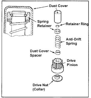
Figure 1. Drive Components, UTE "Bonded" Inertia Drive Starter.
