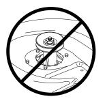
**CAUTION:** Do not allow the customer to operate a mower with any Mandrel safety guards removed.
