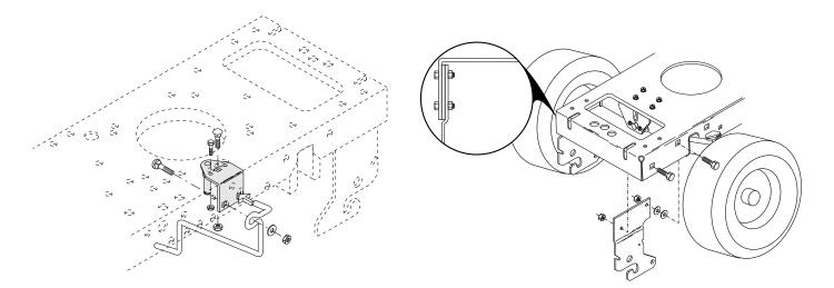
1. LT. tractors - the tractor clutch pedal gets hung up halfway and will not release, causing customer to pull foot pedal back with his toe of shoe to engage drive belt - Solution - drop the tractor motion drive clutch idler assembly and lubricate the idler pin with grease. If the welded pin is rust pitted, you can replace with clutch bracket kit 71/917 #137329
