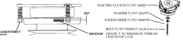
USE LOCKTITE ON THE BOLT TORQUE BOLT TO 50 FT. LB.
