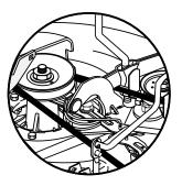
42" mower deck 1995 to 1998 NEW STYLE SUSPENSION TEE PATH BELT ROUTE WITH TWO IDLER PULLEY. USE DECK BELT 71/917 #144200 SIZE 1/2 X 3/8 X 88.38
