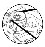
42" mower deck 1994 NEW STYLE SUSPEN-SION TRI-PATH BELT ROUTE WITH ONLY ONE IDLER PULLEY. USE DECK BELT 71/917 #140067 SIZE 1/2 X 11/32 X 86.62
