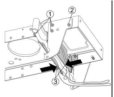
1. LOOSEN FOUR BOLTS HOLDING THE FRONT AXLE BRACES ON RIGHT HAND SIDE OF THE TRACTOR, (ITEM 1), DO NOT LOOSEN BOLT, (ITEM 2).
