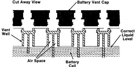
NOTE: Checking the electrolyte is not possible with Maintenance Free Sealed Batteries. If vent plugs are not easily removable, skip this step.
