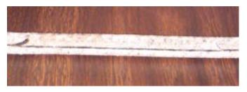
**V-belt Cut from installation by Prying v-belt over pulley** Replace v-belt with <u>correct</u> installation procedure.
