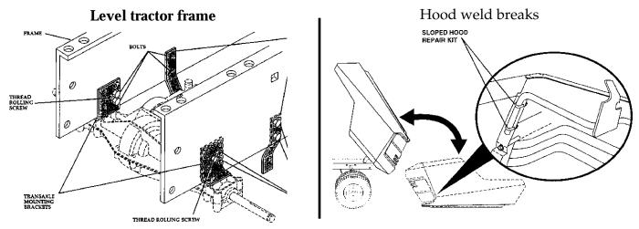
Hood not level on lawn tractor because frame is not level. Solution loosen bolts on transaxle L shape mounting brackets, lift rear of tractor up and down until tractor sits level, retighten bolts.
