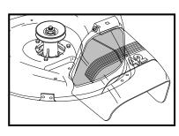
Always mow or mulch grass with the discharge guard attached to the mower deck.
