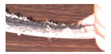
V-belt bottoms out in Pulley or Wear from rough Pulley V-belt worn away at the sides of the 'v'. Check pulley grove and v-belt width. Also check the v-belt pulleys or small rock wedged into the pulley. Worn v-belt sidewalls, v-belt rides at bottom of the pulley grove, replace v-belt and replace damaged 'V' pulley. The pulley groove should not be rough, rusty, or worn.
