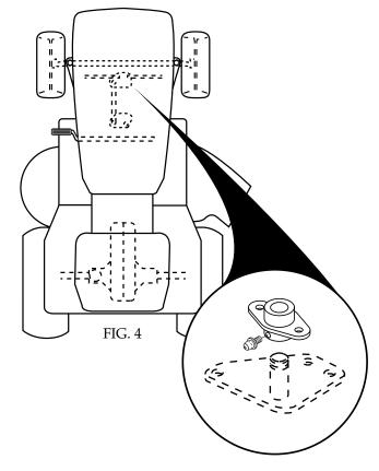
GT. steering on garden tractors with horizontal engine becomes very hard to turn or freezes up - Solution - remove steering bell crank and lubricate the bell crank shaft. Replace bell crank assembly
