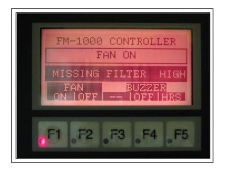
FIGURE 20-1 DISPLAY PANEL MISSING FILTER CONDITION
