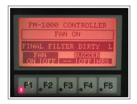
FIGURE 19-1 DISPLAY PANEL FINAL FILTER CONDITION
