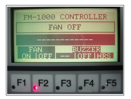
FIGURE 15-1 DISPLAY PANEL FAN OFF CONDITION
