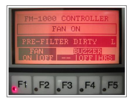
FIGURE 17-1 DISPLAY PANEL DIRTY PRE-FILTER CONDITION
