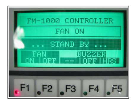
FIGURE 13-1 DISPLAY PANEL FAN ON STAND BY CONDITION
