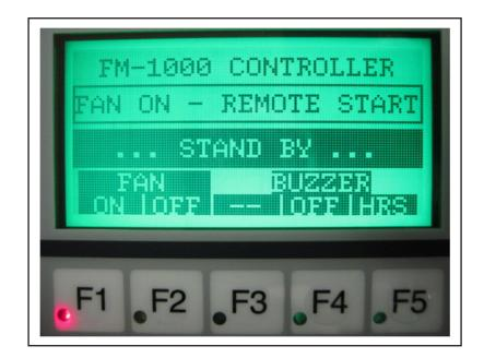
FIGURE 24-1 DISPLAY PANEL REMOTE START CONDITION
