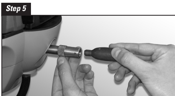
While holding the adapter in place, screw the Quick Clear cartridge into Quick Clear adapter.
