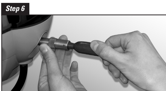
To start cleaning process, while holding Quick Clear Adapter in place, unscrew the Quick Clear cartridge 1/4 Turn Only .
