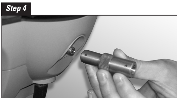
First hand-screw the Quick Clear adapter onto the valve.
