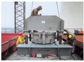
Support bearing and rotor lifting device
