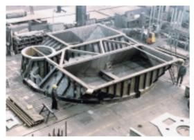
Tri-Sector APH: Workshop assembly of connecting ducts
