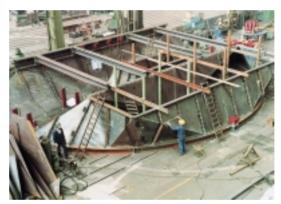
Concentric APH: Manufacturing of connecting ducts
