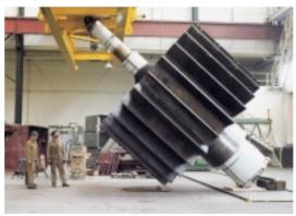
Inner rotor for a large APH before shipping
