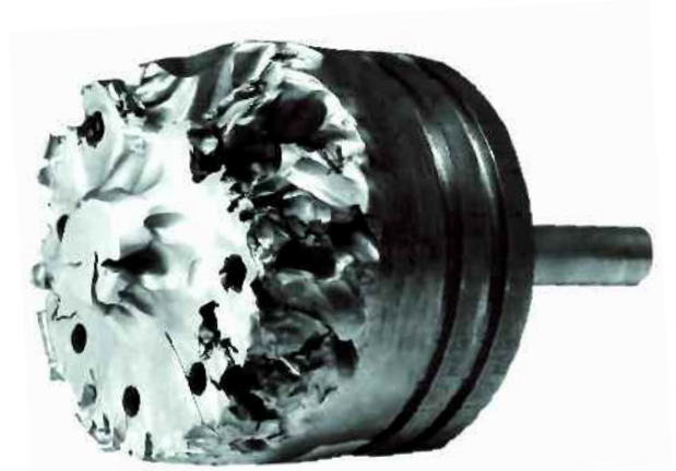
Figure 23. Erosion Damage to Stellite Trim after 2 Weeks Service
