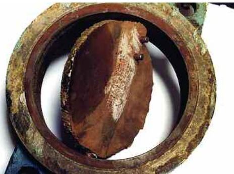
Figure 17. Cavitation Damage to Butterfly Valve
