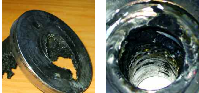
Figure 11. Cage Guided Trim with Severe Cavitation Damage
