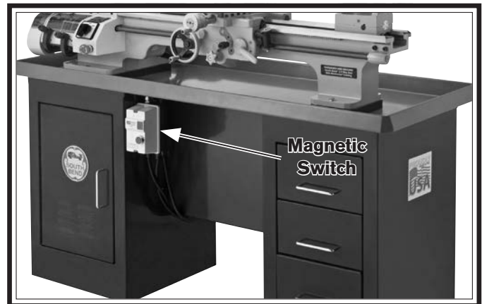
Figure 13. Example photo of the magnetic switch attached to the optional Model SB1035 stand.
