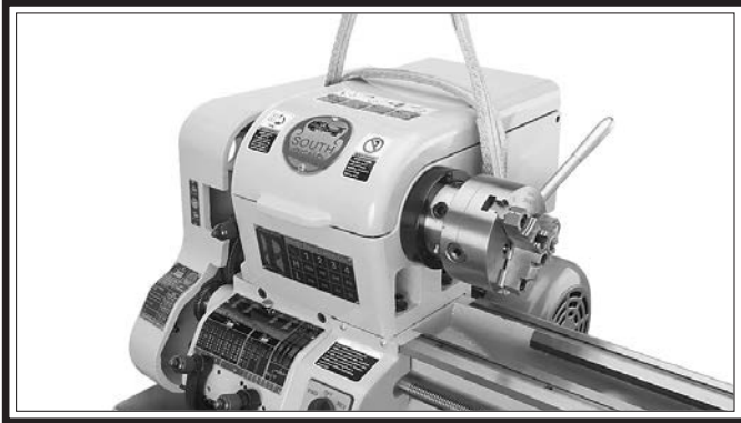
Figure 11. Lifting strap properly positioned through the headstock.
