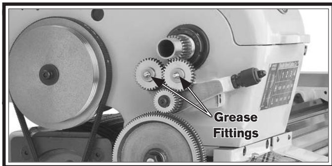
Figure 83. Spindle direction gear grease fittings.
