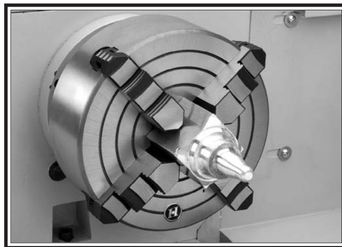
Figure 29. Example photo of non-cylindrical workpiece correctly mounted on the 4-jaw chuck.
