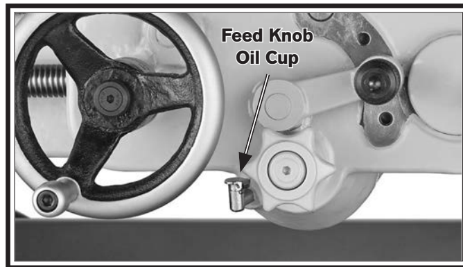
Figure 77. Feed knob oil cup on the apron.
