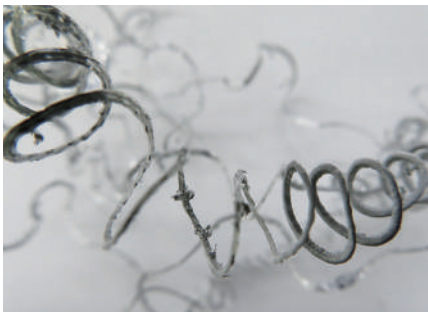
Long chips cause these problems
