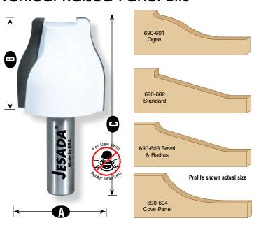
III beautiful raised panel doors and drawer faces with economy and ease! Just use a sturdy fence set 90° to the router table and a minimum 2-1/4 HP router. Maximum safe speed is 18,000 RPM.
