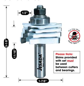
ary the spacing and combinations of cutters to dado, rabbet, tongueand-groove, even slot for biscuits. Our Slot Cutter Set cuts virtually any groove from 1/8" to 11/16", or use any single cutter for precise grooves. Includes 1/8", 5/32", 3/16" & 1/4" carbide-tipped cutters, 1/2" shank arbor, bearing for 1/2"depth-of-cut & shims. For other cutting depths order Depth Adjustment Bearings. Maximum safe operating speed is 18,000 RPM.
