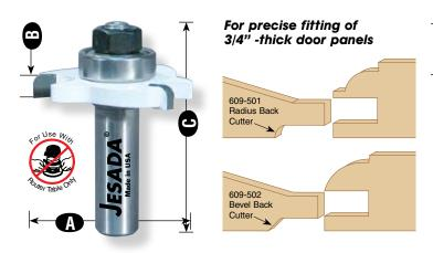
These bits cut a quick rabbet in the back of 3/4" door panels, allowing you to keep the face of the panel flush with the face of the rails & stiles. Just rout the raised panel profile first, then rout the back cut.
