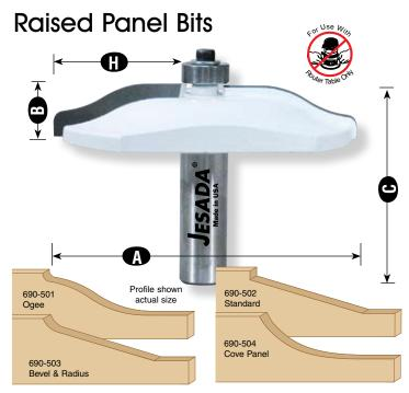
Choose from four popular panel profiles! These bits are perfect for 5/8"-thick door panels. If you're using 3/4" stock, be sure to order one of our new Back Cutter Bits below. Maximum safe speed is 12,000 RPM.
