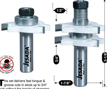
thick without the hassle of changing set-ups for each cut. Cut the grooves with our 1/4" Slot Cutter on a 1/2" arbor, mill the tongue with a pair of 1/4" cutters mounted on a separate 1/2" arbor. Maximum safe speed is 18,000 RPM.
