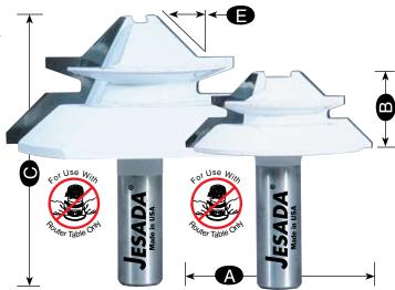
These bits cut the strongest miter joints you'll ever use. Use the Lock Miter Bit (655-503) with stock from 5/8" to 1-1/8" thick or use the Lock Miter "Junior" (655-502) for stock from 3/8" to 11/16" thick. Build boxes, frames, beams, face-frame corners and many other right-angle joints. Maximum safe speed is 16,000 RPM.
