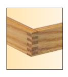
ox joints are beautiful a strong-they're also fast & easy with this bit. The bit includes five 5/32" slot cutters mounted on a 1/2" arbor, allowing you to make 5/32" combs in stock up to 1-9/16" high (up to 3-1/8" in 2 passes). Also includes a bearing for 1/2" depth of cut, use your fence for shallower cuts. Works with stock up to 1/2" thick.
