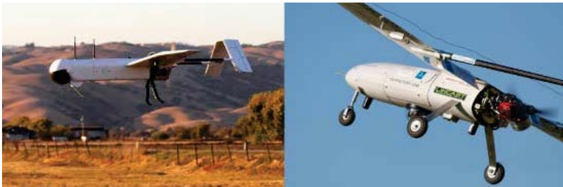
Figure D - 20 - Fixed Wing UAS with Skid Landing Gear (left); Standard Landing Gear (right)
