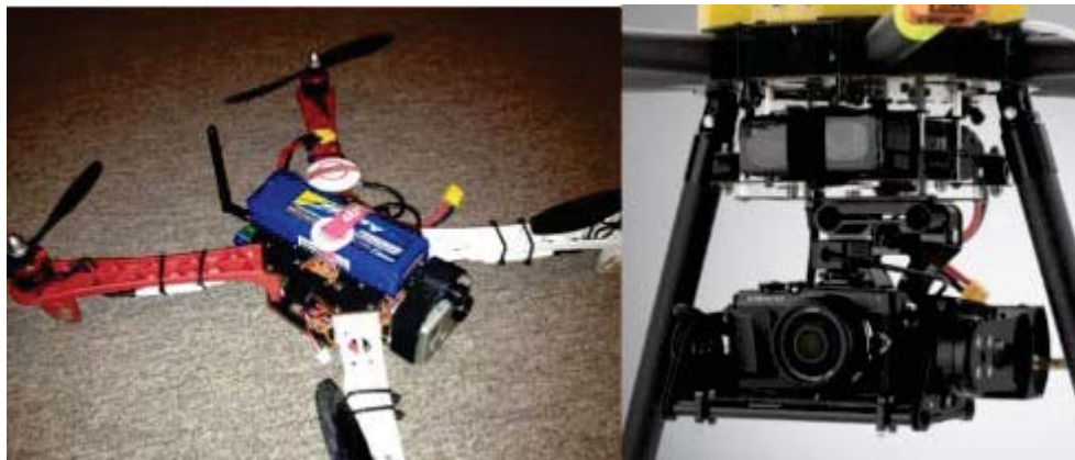
Figure D - 14 - Battery Mounted above Main Body with Velcro (left); Battery Mounted Below Main Body (right)
