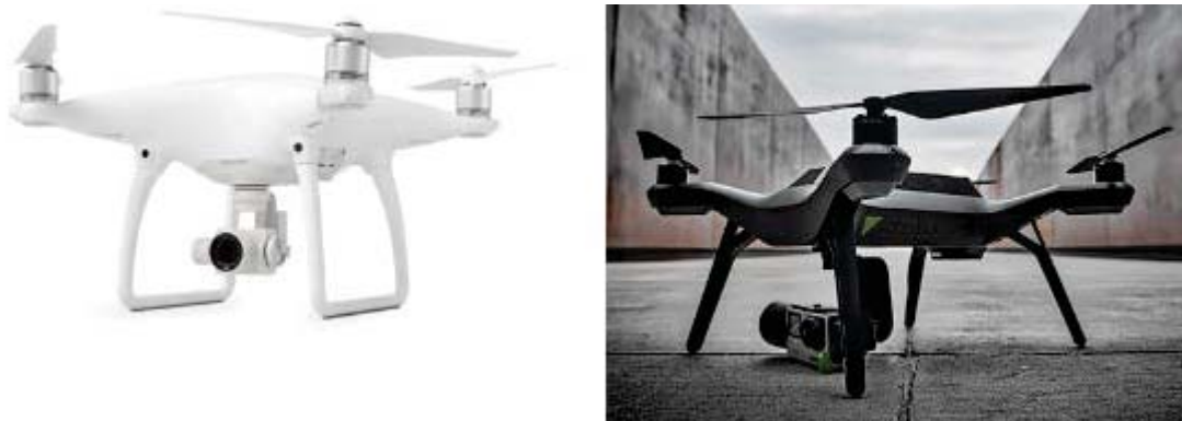
Figure D - 6 - Smooth Contours on Fuselage (DJI Phantom on left); Sharp Edges on Fuselage (3DR Solo on right)
