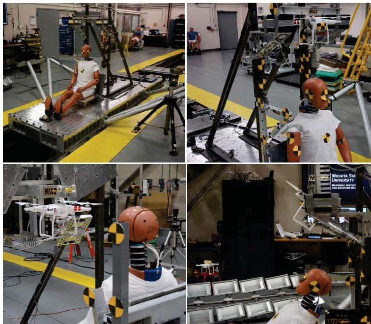
Figure 18 - Front Left View of Sled Setup (upper left), Vertical Drop Position of Dummy and UAS (upper right), Pendulum Setup for Horizontal Impact Test (lower left), and Dummy and UAS Setup for Angle Impact Test (lower right)
