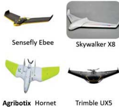
Figure D - 3 - Fixed Wing UAS with Flying Wing Configuration
