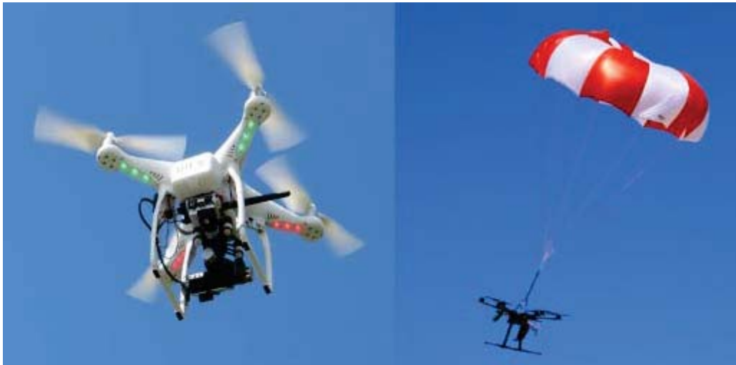
Figure D - 25 - Visual Warning Systems on Multirotor UAS (left); Parachutes on Multirotor UAS (right)
