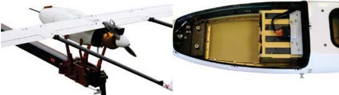
Figure D - 16 - Rear-Mounted Engine on a 50 lbs UAS (left); LiPo Batteries inside the Fuselage of a 33 lbs UAS (right)
