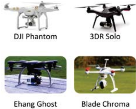
Figure D - 1 - Multi-Rotor UAS with Monocoque Body Construction
