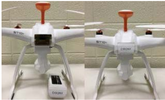
Figure D - 13 - Smart Battery and Internal Compartment (left) Battery Held Firmly inside Fuselage (right)
