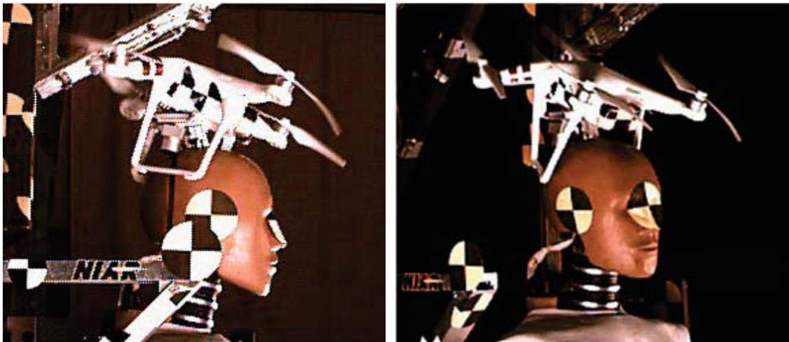
Figure 45 - Phantom 3 Standard Fuselage Deformation During NIAR 50-foot Drop Test Impacts (Test UA17A-13)
