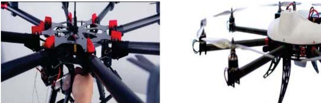
Figure D - 7 - Sharp edges on Fuselage main body (left); Plastic casing on the main body (right)
