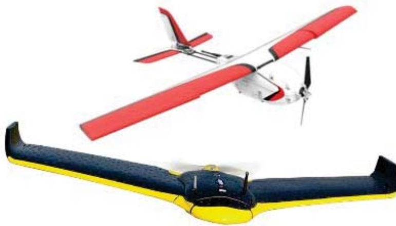
Figure D - 9 - Fixed wing UAS with conical-shaped fuselage and fore-mounted engine/propellers (Upper Red/White aircraft); Rounded Leading Edge and Nose Cone (Lower Black and Yellow aircraft)
