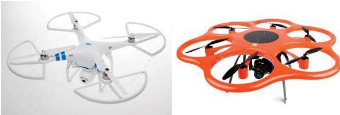
Figure D - 11 - Propeller Guards (left); Shrouded Propellers (right)
