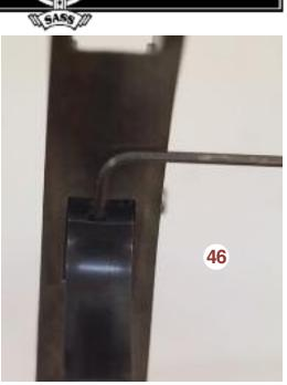
push in the safety bar and pull the trigger until the lower adjusting screw is visible in the front of the trigger. **Photo 45.** Insert the Allen wrench (try using the short end of the Allen wrench as it provides more clearance for this screw) and adjust the forward travel of the trigger. **Photo 46.** You want to adjust the trigger so that when the trigger is pulled the sear tip just <u>(Continued on page 44)</u>
