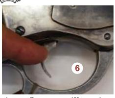
piece trigger and eliminate trigger flop, yet still retain the trigger safety. To install the trigger, the action has to be completely disassembled. Remove the stock, the slide plates and all the internal parts. This is as far as most people go for routine maintenance of their
