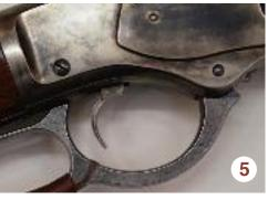
used a two-piece trigger, with the sear being able to pivot independently from the trigger. This creates a problem for speed tuning a modern 73 for SASS competition. **Photo 5** shows the trigger at its rearward position. **Photo 6** shows the trigger at its forward position. On this particular gun there is almost 3/8ths of an inch of trigger flop at the tip of the trigger.
