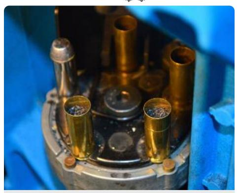
Here 35 grains of Goex Cartridge is loaded under 200-grain bullets in .45 Colt cases. This is a slightly compressed load.
