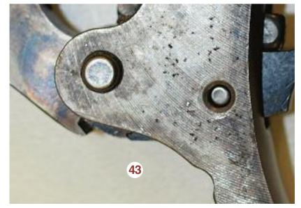
two trigger screws on the front of the trigger become visible. **Photo 42.** Insert the Allen wrench into the UPPER screw and adjust sear engagement. **Photo 43** shows the sear fully engaged in the full cock notch. (Continued on next page)
