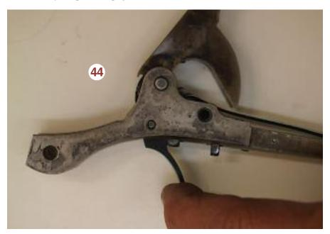
(The large notch higher up on the hammer is the half cock notch.) After sear engagement is set, pull the trigger to make sure the safety bar stops the trigger and the hammer does not fall. **Photo 44.** If the hammer falls, readjust the sear and/or trigger rear travel screw(s) until everything operates properly. Finally,
