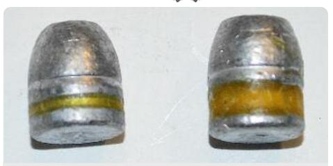
200-grain RNFP .45 Colt bullets. The one on the left has normal smokeless-sized lube grooves. The one on the right has a Big Lube groove to hold enough lube for shooting black powder in rifles.
