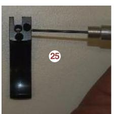
hole from the FRONT of the trigger. Photo 24. The upper hole on the right, Photo 25, is for adjusting how far the trigger can travel forward.
