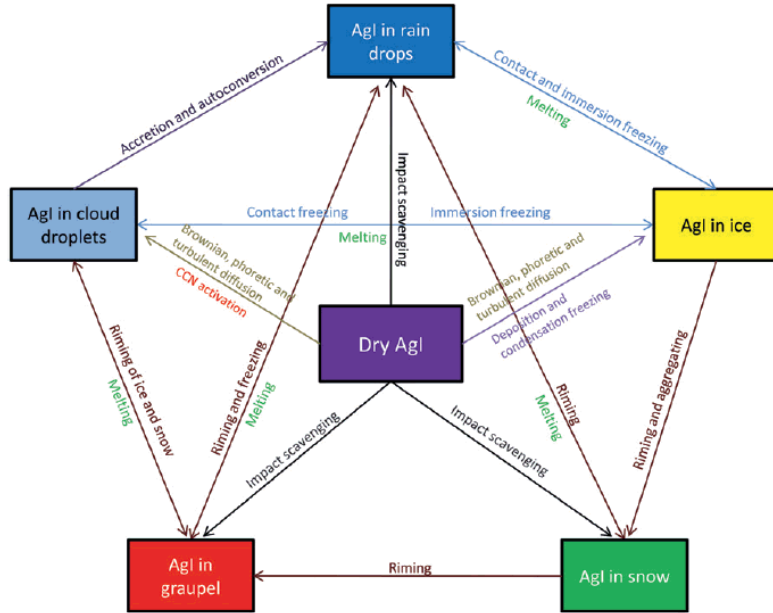
Figure 3.23 AgI parameterization logic used in the WRF model as described by Xue, 2013a
