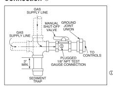
Manual shut-off valve is in the "OFF" position when handle is perpendicular
