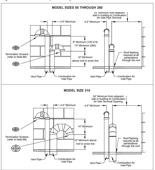
Figure 9.2 - Vertical 2-Pipe Vent System for Sloped Roofs
