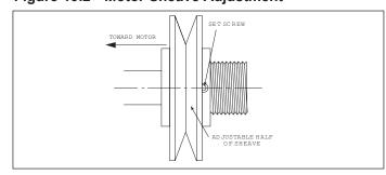
Figure 19.3 - Belt Tension Adjustment
