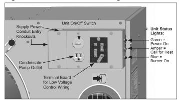
All supply power electrical connections are made in the junction box compartment of the unit. The low voltage (thermostat and accessory control devices) can be wired to the terminals on the junction box.
