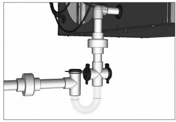
Figure 13.3 - Vacuum Breaker Example
