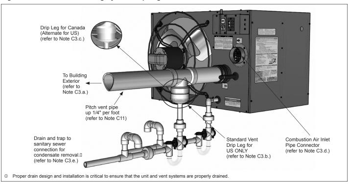
Figure 11.1 - Horizontal 2-Pipe Vent System
