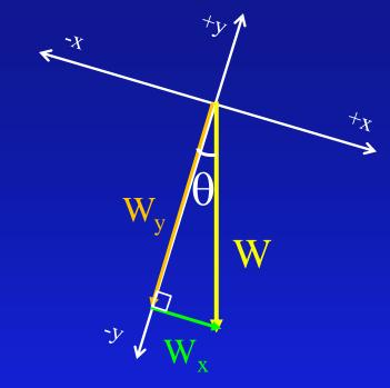
Split W into COMPONENTS parallel to axes
