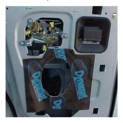
The new speaker is in, after installing the Dynamat and replacing the factory plastic barrier. To help align the barrier sheet, note that there are two little bumps in the sheet metal (at the top corners) that line up with holes in the barrier.
