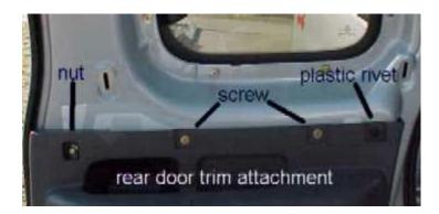
Now, just lift up to release the tabs and the panel pulls away. Don't try to pull out on the panel until you have lifted in up enough to completely disengage the tabs (i.e. don't force it).
