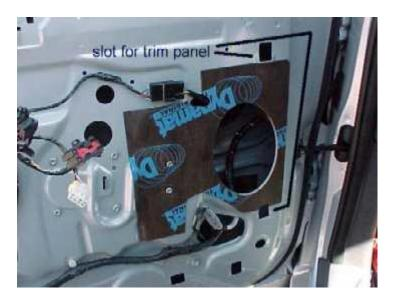
Here is the completed installation showing the speaker installed over the replaced factory insulation sheet. As before, everything goes back in the reverse of the disassembly. Don't forget to replace the marker light socket, and be careful to get the door lock knob through the hole. It may help to pull the knob up first.
