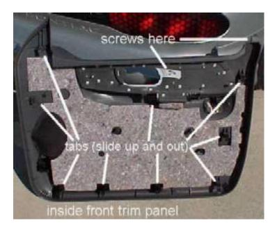
Again, I removed the factory barrier/insulation in order to install the Dynamat. I also stuck the part cut out for the speaker to the inside of the outside skin.
