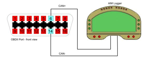
Warning :OBDII is not powered by the vehicle master switch, so if AIM logger is connected to OBDII for a long time the battery runs down. The communication works only if the dashboard is switched on.
