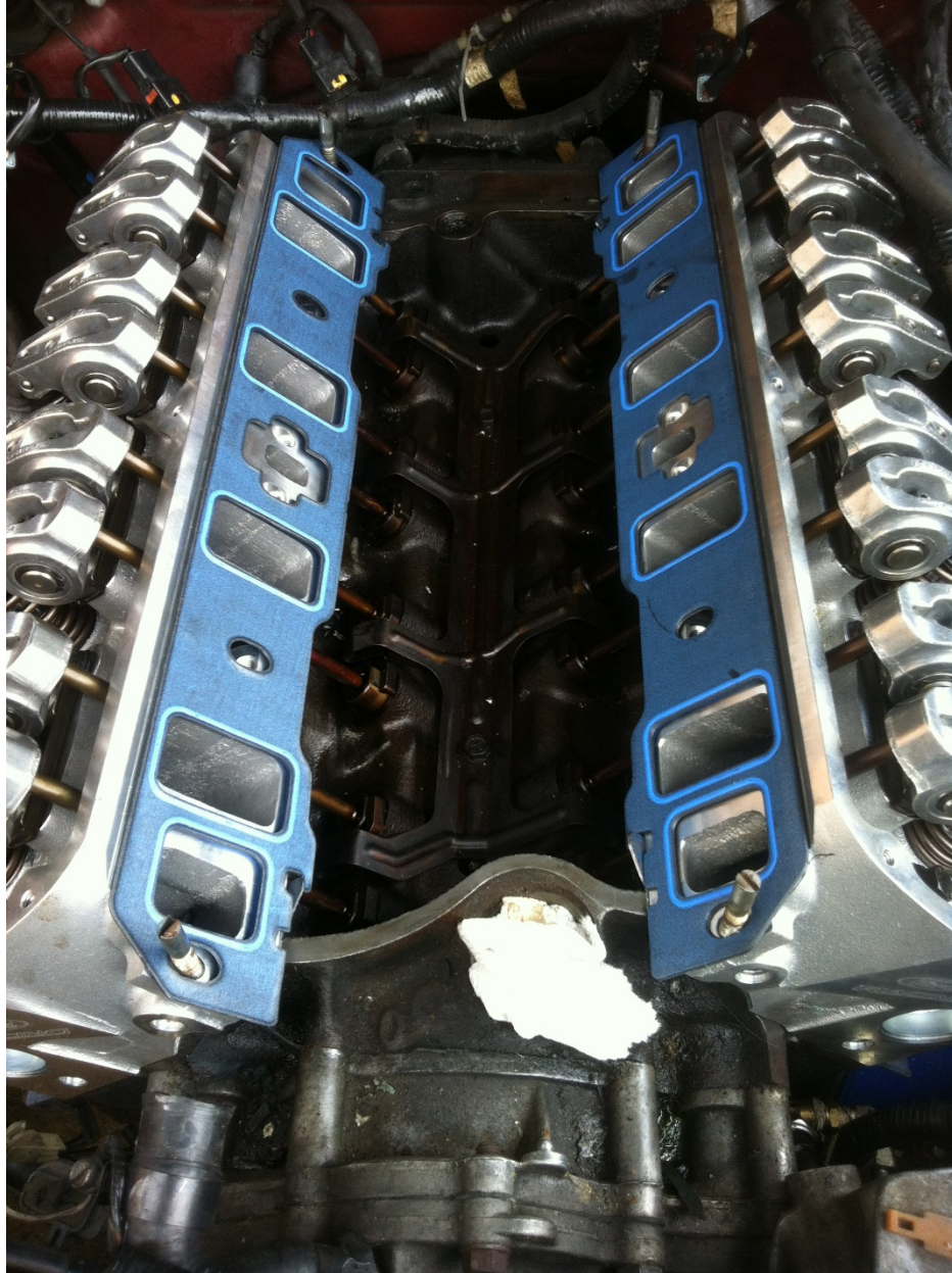
Step 56. Photo 24: Always check port alignment of your gaskets between the cylinder head and intake.
