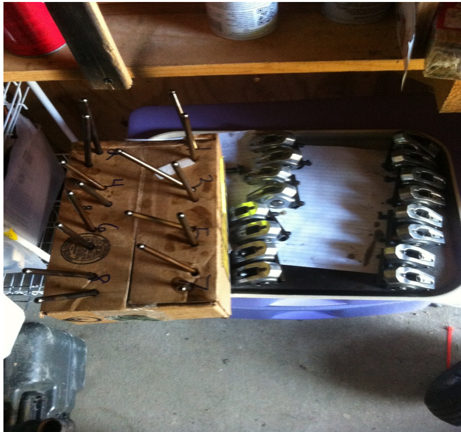
Step 35. Photo 14: Keeping track of location of valvetrain components (if reusing them) to ensure they go back in same locations during reassembly.
