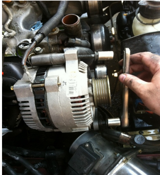
Step 28. Photo 10: Removal of alternator from accessory bracket.
