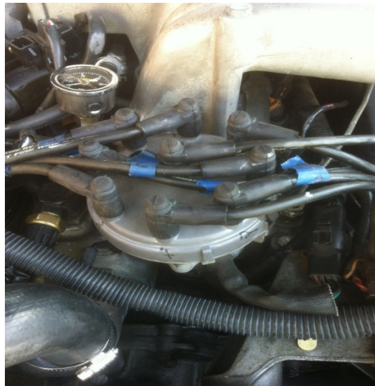
Step 23. Photo 8: Labeling distributor cap and plug wires for convenience later on.
