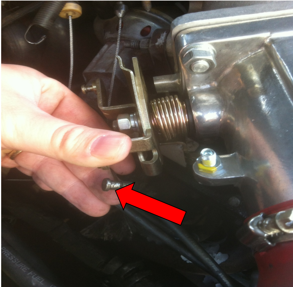
Step 7. Photo 1: Rotating throttle to remove cable.
