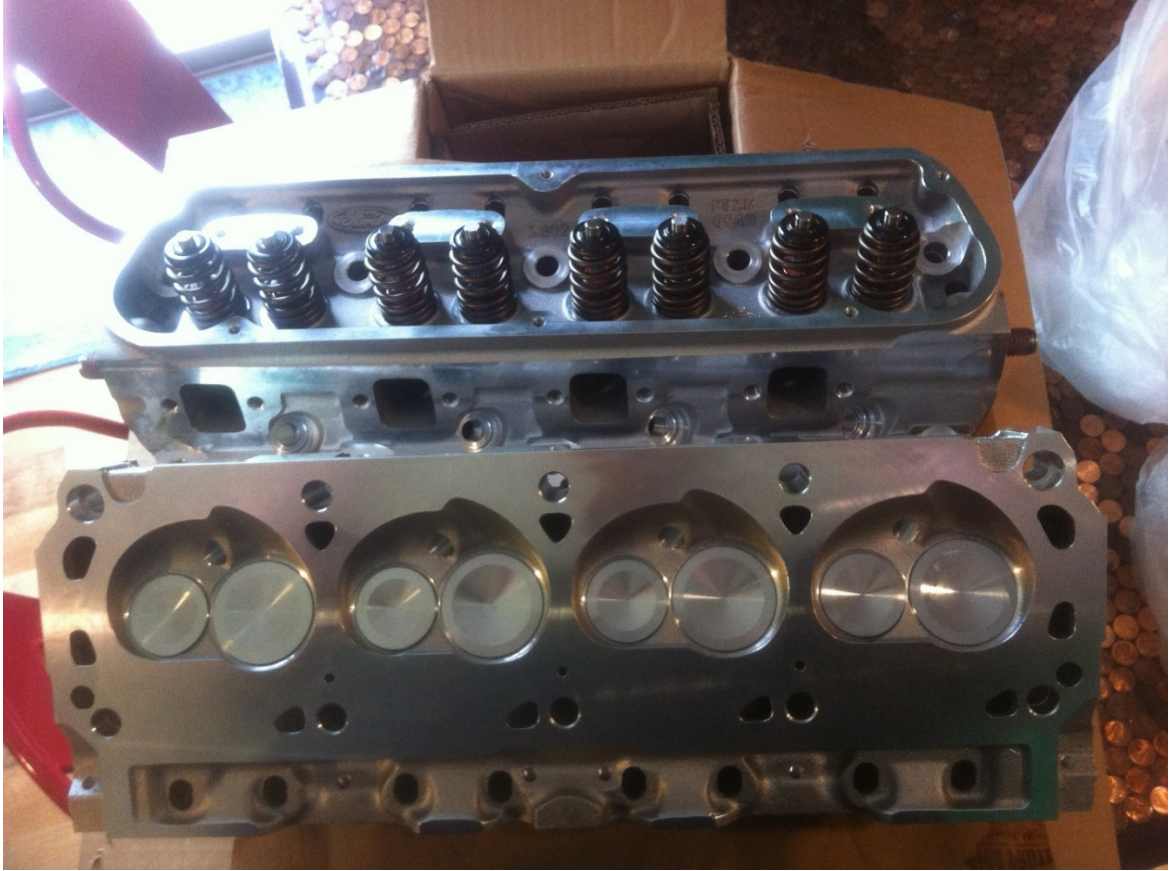
Step 39. Photo 16a: Unboxing New GT40X cylinder heads.
