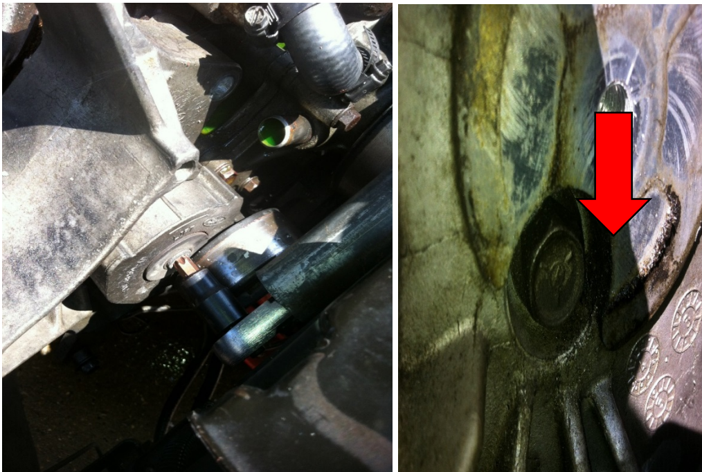
Step 29. Photo 11: Use Torx T-45 to remove belt tensioner to expose bolt underneath to remove accessory bracket from passenger cylinder head 94-95' models (Fox similar).
