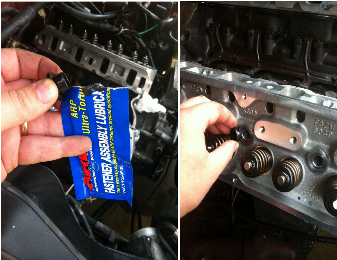
Step 45. Photo 19: Applying assembly lube to step washer and mounting on cylinder heads.
