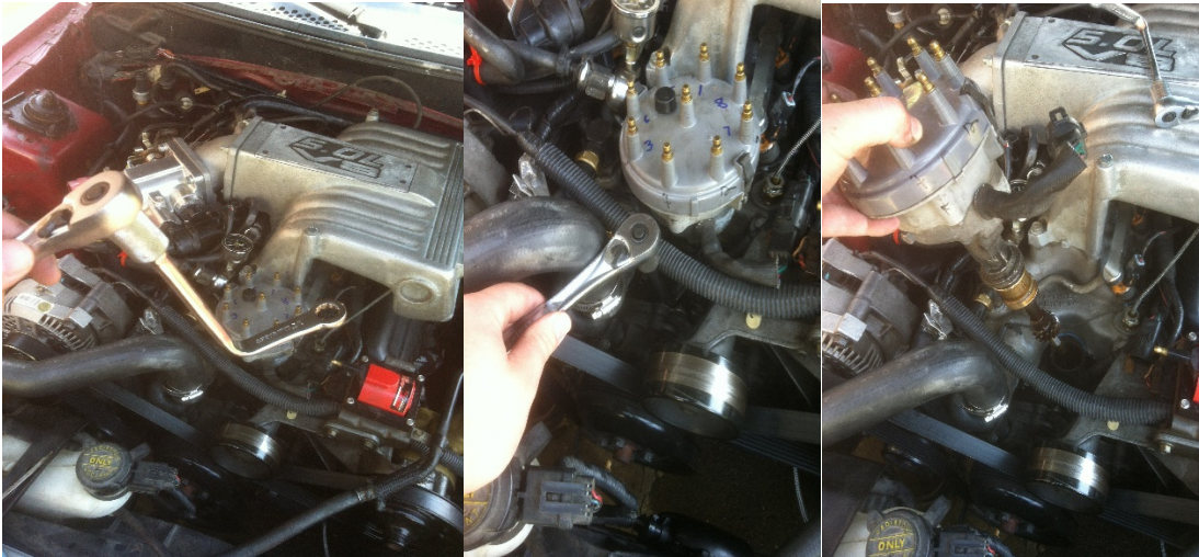
Step 24. Photo 9: Using distributor wrench to remove \frac{1}{2} " bolt securing distributor.
