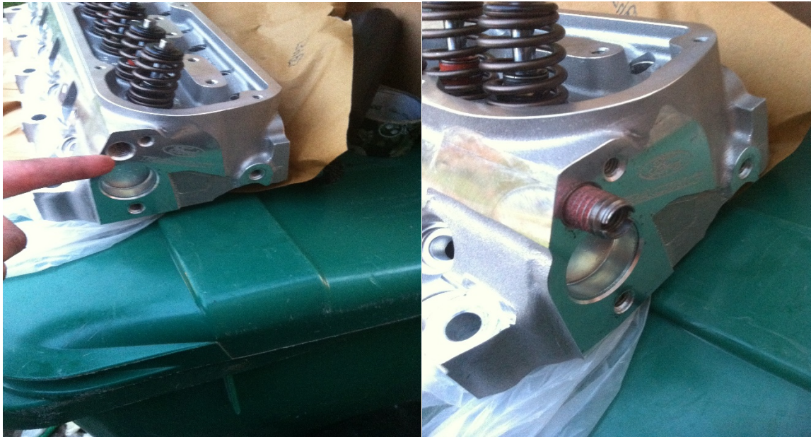
Step 39. Photo 16b: Installing cylinder head plugs in correct side for installation.
