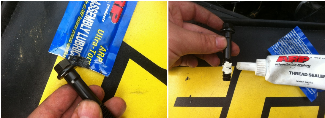
Step 46/47. Photo 20: Preparing head bolts with assembly lube and thread sealer for the short bolts that will be in the water jackets.
