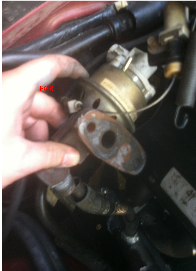
Step 11. Photo 2: 94-95' Models have EGR plumbed directly into passenger exhaust manifold.
