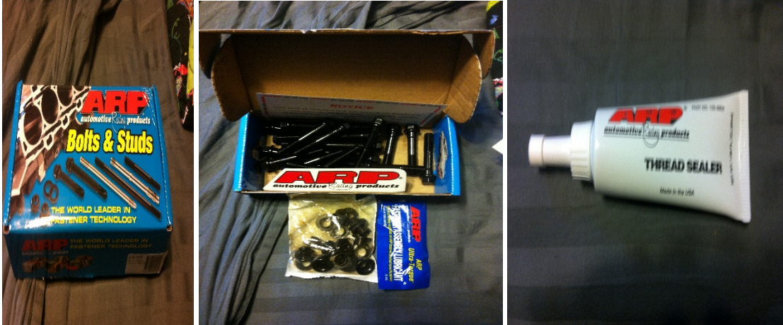
Ford Racing (ARP) 289/302 head bolt kit Item # 50146 and ARP thread sealant (Item # 18221)
