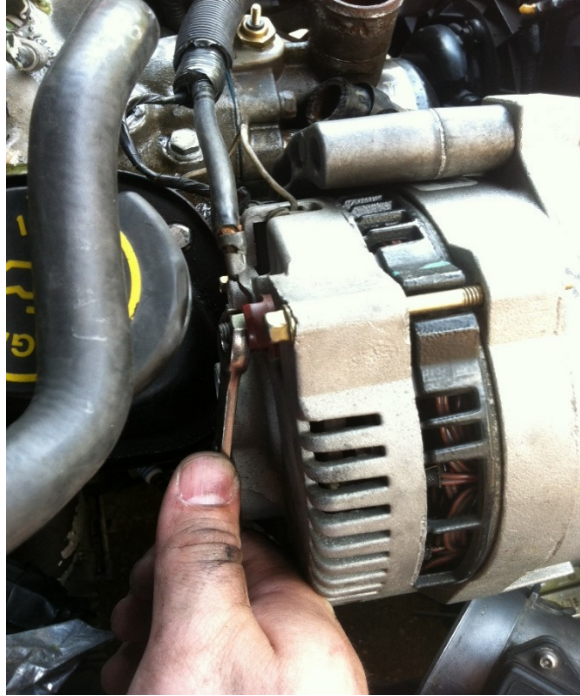
Step 22. Photo 7: Removal of alternator wiring 94-95' models (Fox similar).
