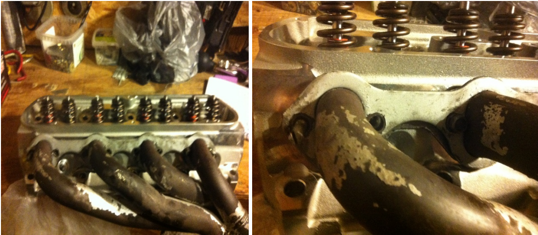
Step 40/41. Photo 17: Pre-installing headers and checking for port matching. Make sure you can access the shorter head bolts before mounting headers, in my case the passenger side I had to install the header after the head was torqued down.
