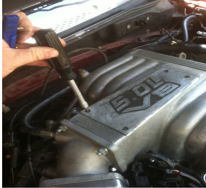
Step 13. Photo 3: Torx T-20 for plenum cover. 6 bolts (1/2") secure upper plenum to lower.
