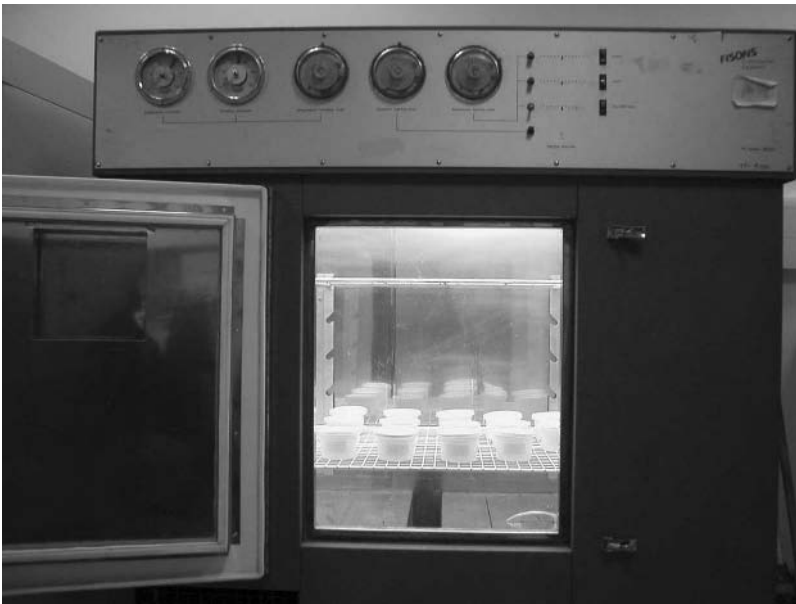
Figure 6.1 Larvae collected from the crime scene are reared in a controlled environment cabinet. They are kept in pots
