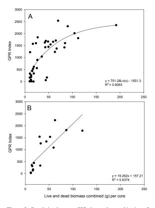
**Figure 8.** Correlation between GPR data and a combination of both live and dead biomass. Inset A includes all data from the 40 cores sampled at Sanderson PPINES in 2005, Inset B reduces the 5 cores collected in each transect to 2 classifications (bed and inter-bed) resulting in 16 data points. If inset A were fitted with a linear equation the R<sup>2</sup> would equal 0.50.
