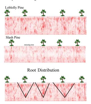
Figure 4. Examples of data collected at the IMPAC site, the tree locations are denoted by the small "tree" graphic. The upper two scans demonstrate differences between species, while the bottom scan illustrates root distribution (0-50 cm depth scale) along a transect.
