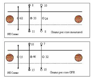
Figure 7. Compare actual root mass collected from soil cores and estimates from GPR for each core position across all families/spacing.
