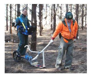
**Figure 1.** SIR 2000 Ground-penetrating radar system used with a forest survey rig, compromised of a high-frequency GPR antenna mounted on a stabilization board (1.5 GHz) and a survey wheel.
