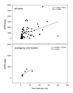
Figure 6. The correlation coefficient of GPR data and root mass individual root cores (all cores) was small at the Sanderson PPINES site, when the average values of GPR index and root mass were correlated for each core position (Figure 3) the  $R^2$  value improved.
