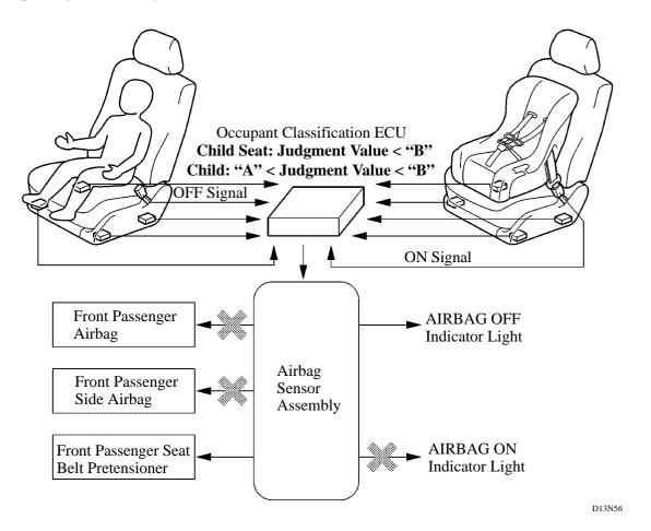
After the occupant classification ECU judges that child seat is installed, the AIRBAG OFF indicator light does not go OFF unless the seat belt buckle switch is turned OFF.
