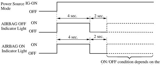
ON/OFF condition depends on the front passenger detection result. 259ESW53
