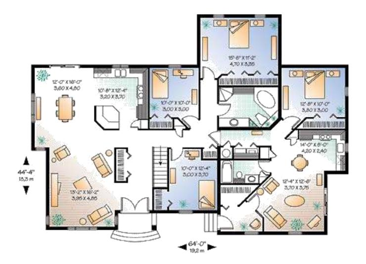
This type of drawing shows the layout of the rooms inside the building and the position of the doors, windows and important fittings like a bath, sink and toilet.
