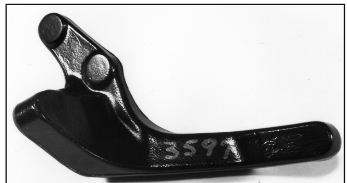
The forged microalloyed steel engine mount has a complex geometry. It provided the required property profile using a ferrite pearlite microstructure.
