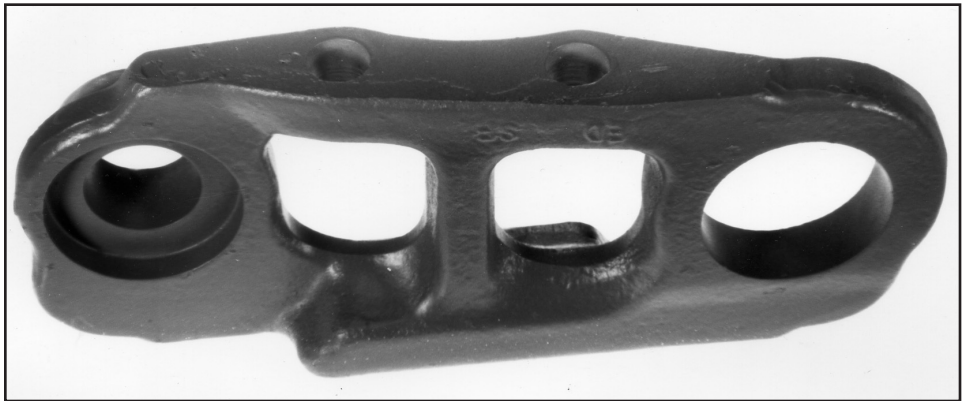
The hardened and tempered track link featured an induction hardened rail section (at the bottom of the part) that provided higher wear resistance.
