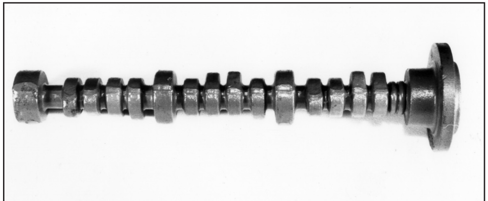
Approximately 15.5 in. long with a 3.75 in. hub diameter, the forged 5150 steel camshaft was used on a fuel injected 3.8 L engine.
