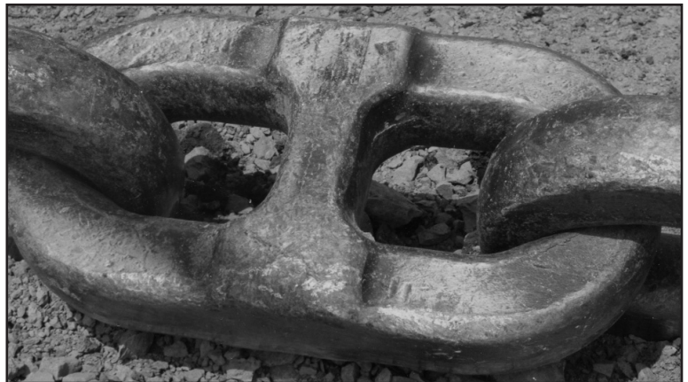
Forged in a series of sequential dies on a counterblow hammer, the dragline chain links delivered mechanical properties and performance that surpass other methods of manufacture. The link is 5.25 in. thick, 50 in. long and 26 in. wide, and it weighs 1375 lbs.
