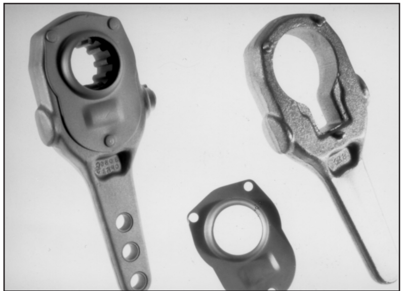
The forged slack adjuster was made from high carbon steel, which was resulfurized for improved machinability. It contained integral lugs that outperformed both pin riveted and spot-welded assemblies.
