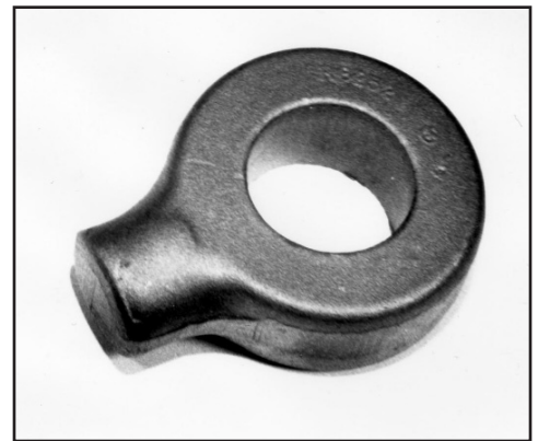
Forged from 1045 steel, the rod end needed only an inexpensive broaching operation prior to being friction welded to a shaft.
