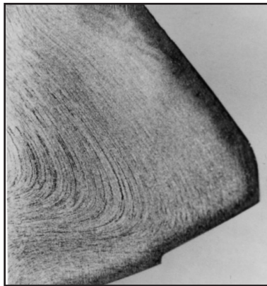
Grain flow that follows the contour of forged teeth in steel bevel gears is directly responsible for improvements in fatigue life over machined gears.
