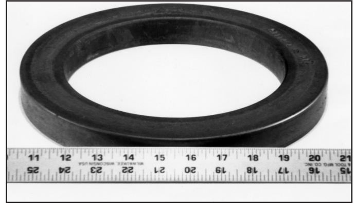
Rolled steel rings have replaced more costly heavy wall tubing, which was cut to shape and contoured into ring gears.
