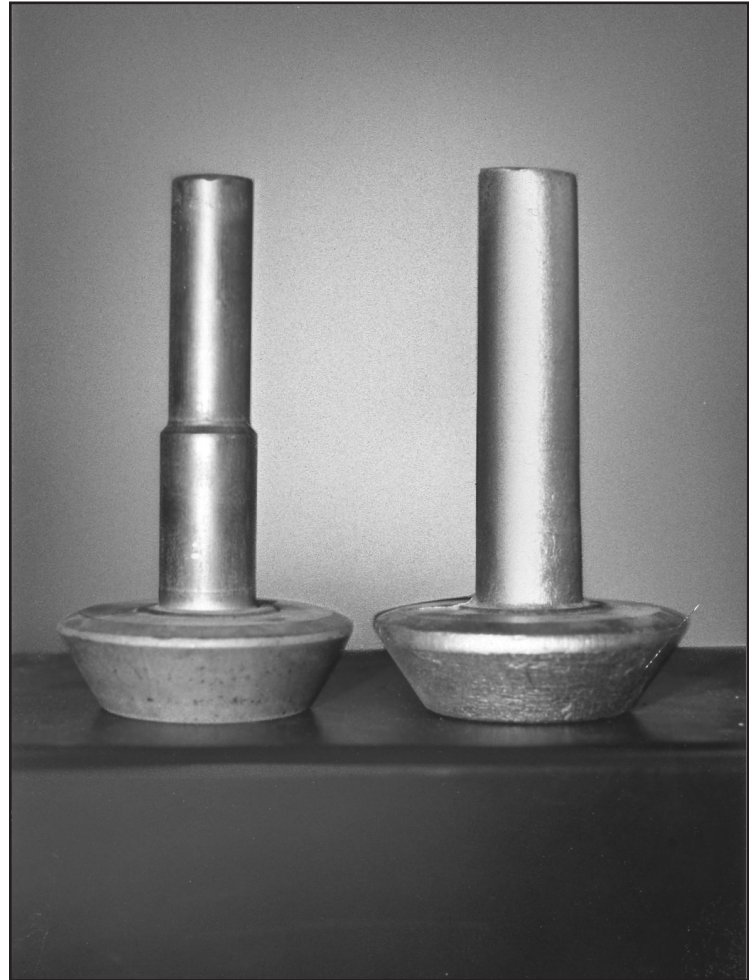
Warm forged automotive drive pinion (left) is produced closer to net shape than a hot forged version (right), saving material and energy and reducing required machining.
