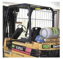
An overhead guard can deflect objects falling from above.
