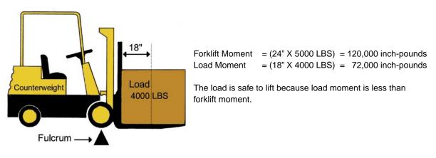
However if the 4000 pound load was 66" wide, the load moment would be  $(33" \times 4000 \text{ lb.}) = 132,000$  inch-pounds which would be greater than the moment of the forklift. The forklift would tip forward.
