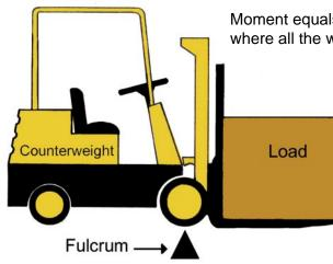
Example: an evenly distributed 36" wide load on the forks has a center of gravity that is 18" from the face of the forks<sup>1</sup>. If the load weighs 4000 pounds then the load moment will be  $(18" \times 4000 \text{ lb.}) = 72,000 \text{ inch-pounds}$ .
