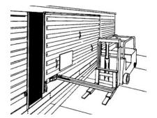
Forklift attachment used to open railroad car doors.
