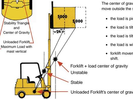
The center of gravity of the forklift-load combination can move outside the stability triangle if:
