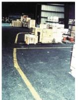
Mark aisles to help keep adequate clearance for forklifts.
