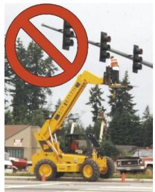
Never stand on the forks or a pallet to work at an elevated level.
