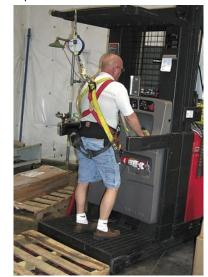
The operator of an order picker type forklift must wear a safety harness to protect against the fall hazard at an eleveated location.
