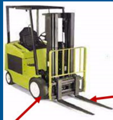
Forks on a forklift. Some trucks have a solid platform and are called "platform trucks".
