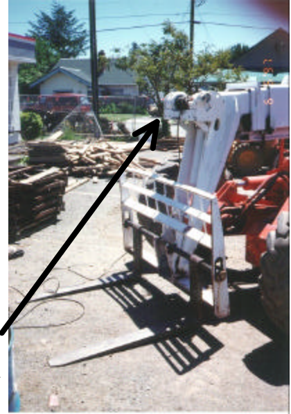
A winch was welded on the boom of this telescoping truck without the manufacturer's approval.
