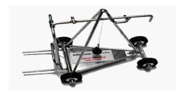
This model demonstrates how forklifts have a three point suspension and illustrates the stability triangle.
