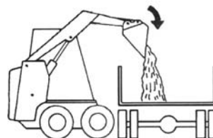
Fig. 25: Dumping Into a Box
