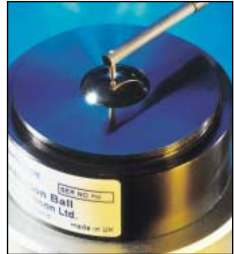
calibration over a ball checks stylus condition, gauge range, linearity and processor functions
