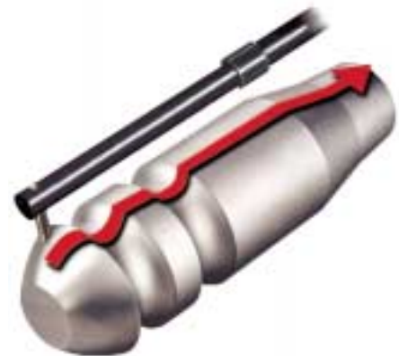
measuring path for raw profile
