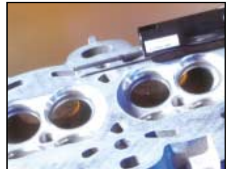
high resolution skidless pick-up is necessary for straightness and waviness measurements
