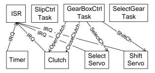
*Figure* 7.6 Model overview – timed automata (rectangles) and synchronizations via channels (arrows)
