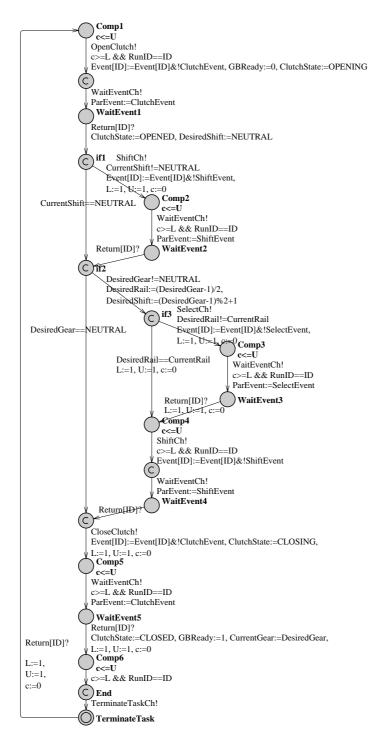
Figure 7.13 GearBoxCtrlTask timed automaton
