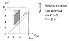
Figure 6.1 Possible values of relative finishing time  $F_T$  of the interrupted computation of the task T versus the ISR execution time  $C_{ISR}$
