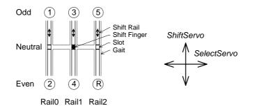
Figure 7.1 Gear box mechanism
