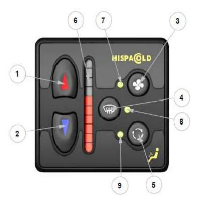
The control consists of 5 keys for the selection of the different functions, a bar of leds for the indication of the temperature level required and three leds or light indicators to signal the activation of the different elements.
