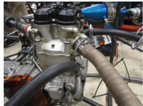
Inlet and outlet hoses into engine from radiator
