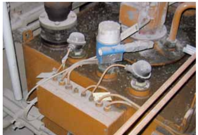
Liquicap maintains level in lubrication oil surge tank
