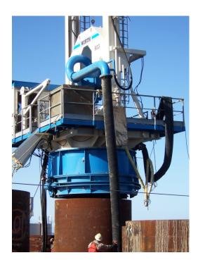
Figure 6-12. Reverse Circulation Drilling Equipment.
