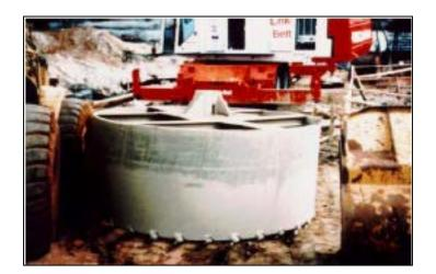
Figure 6-8. Core Barrel.
