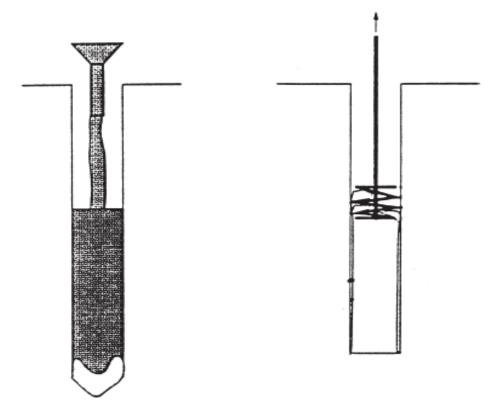
Figure 6-17. Pile Defects - No Cleanout, Tapered Bottom of Hole.
