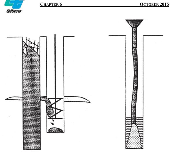
Figure 6-21. Pile Defects–Adjacent Hole Blowout.
