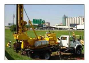
Figure 6-15. Truck Mounted Drill Rig.
