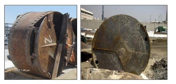
Figure 6-6. Drilling Bucket.
