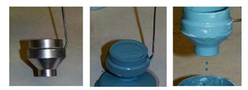
Figure 8. Measurement of viscosity with a flow cup [45].
