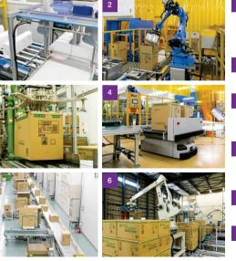
After cutting, products are packed into plastic bags by the automatic packaging machine. Then, they are transported automatically by conveyor
