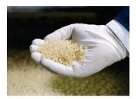
Our production plants in Kanto, Chubu, and Fukuyama have recycling centers. There, used containers are collected from across Japan and eco-friendly products are manufactured using recycled materials. The photo at left shows the pellets recycled from used containers.
