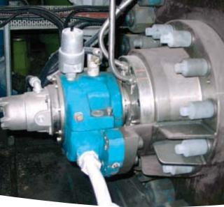
Balance valve and thrust bearing housing upgrades extend the life of between bearings pumps
