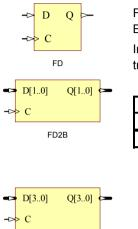
FD, FD2, FD4, FD8, FD16, FD32 are, respectively 1-, 2-, 4-, 8-, 16-, 32-Bit D-type positive edge trigger flip-flop.
