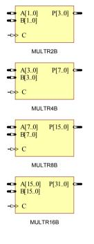
MULTR2, MULTR4, MULTR8, MULTR16, MULTR18, MULTR32 are respectively 2x2, 4x4, 8x8, 16x16, 18x18, 32x32 registered signed multipliers. They perform multiplication of two signed values from the two inputs (A and B) on the rising-edge of the clock input (C) and produce a product (P).
