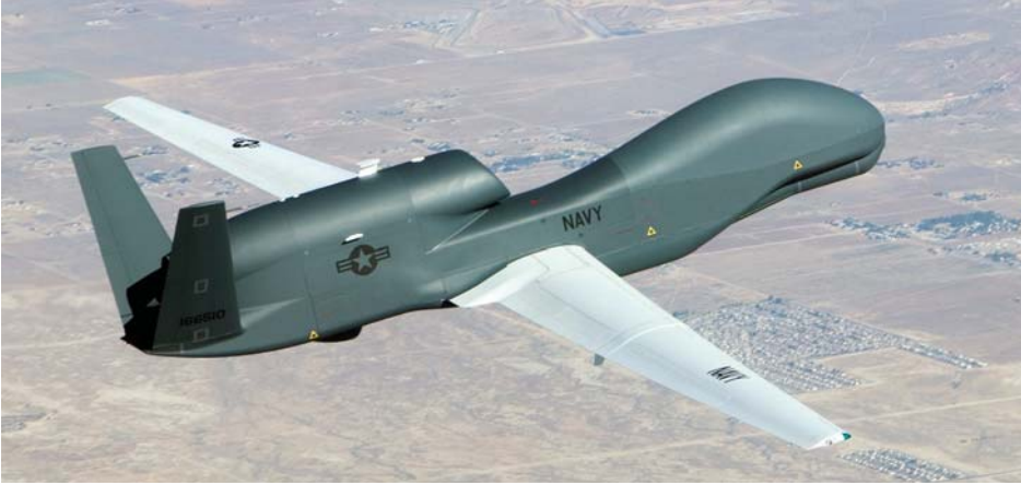
Figure 2 – The Global Hawk unmanned aerial vehicle typically flies reconnaissance missions at 60,000 feet and can refuel in midair to stay aloft many days at a time. It is one of a growing armada of unmanned vehicles remotely controlled via the GIG.
