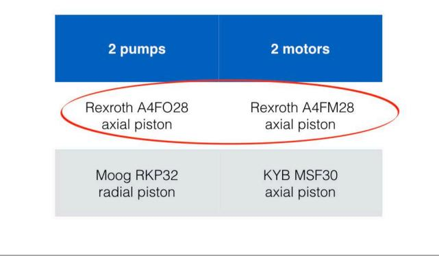
The pumps are an axial piston slipper type machine, and a radial piston pump.
