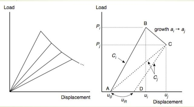
Left: load displacement curve for elastic fracture where the test is periodically stopped and unloaded. Right: A single loading and unloading envelop. Elastic fracture follows path ABC. Fracture with residual displacements follows path ABCD.
