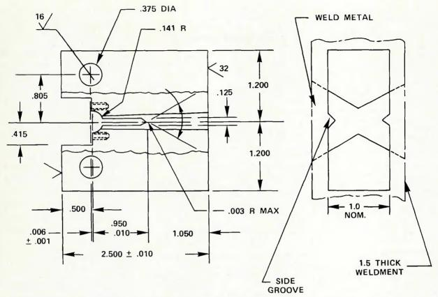
Fig. 1—Modified compact specimen (1TCT) for J-integral testing. Dimensions are shown in inches (1 in. = 25.4 mm)
