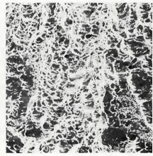
Fig. 4—SEM fractographs of GTA weld metals: Left—HY-130/AB; Right—HY-130/Y
