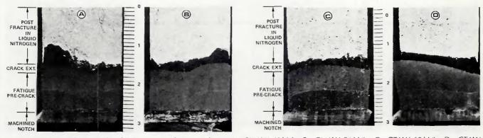
Fig. 2 — Typical macroiractographs of J<sub>IC</sub> fracture toughness specimens: A — GMAW, 46 kJ/in.; B — GMAW, 81 kJ/in.; C — GTAW, 65 kJ/in.; D — GTAW, 34 kJ/in.
