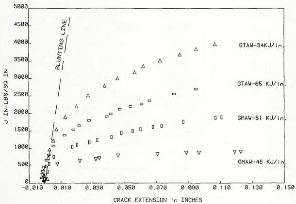
Fig. 3-J vs. crack extension of HY-130 welds
