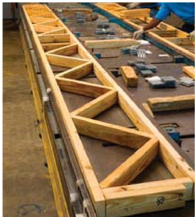
(Fig. 19) Trusses are assembled in a manufacturing plant.
