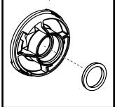
\*\* It is important that the nozzle seal inside the nozzle be re-installed properly. Make sure the cup side of the seal (the side with the groove) is facing out towards the front of the nozzle. Improper installation will cause leakage and damage to the turbine.
