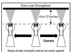
When spraying, always trigger the spray gun after spray pass has begun and release trigger before stopping the pass. Always keep the gun pointed squarely at the spray surface and overlap passes slightly to obtain the most consistent and professional finish possible.
