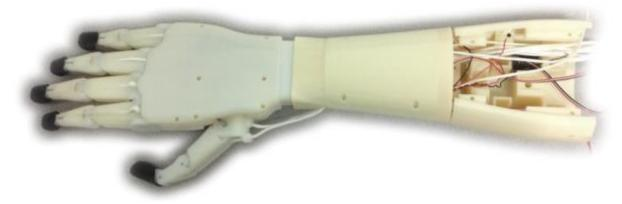
Figure 7: IRIS Cable Operated Prosthetic Device
