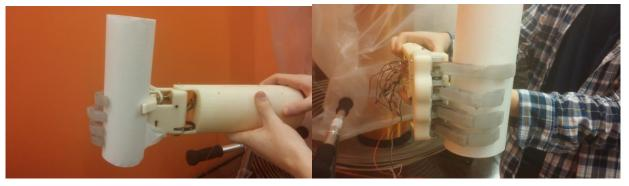
Figure 26: Holding the Heavier and Harder to Grip Paper Towel Roll
