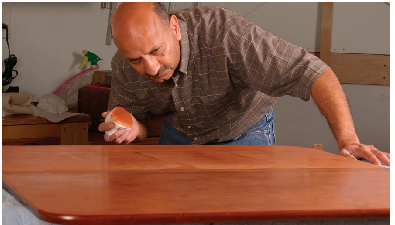
Pounce the pumice. Pour some superfine 4F pumice into a cotton bag and then knock the bag at even intervals on the workpiece.
