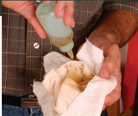
Prepare the pad. The pad consists of a cotton batting core inside a linen covering. Dampen the core with very dilute shellac.
