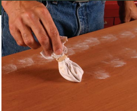
Pounce the pumice. Pour some superfine 4F pumice into a cotton bag and then knock the bag at even intervals on the workpiece.
