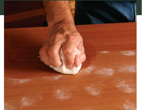
Fill the grain. Force the pumice into the wood's pores using a circular motion. Sprinkle on more pumice until the pores are filled.
