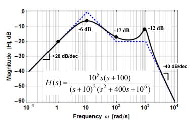
Figure 1-12 – Example problem integrating many common features of Bode plots.
