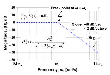
Figure 1-7 – Uncorrected Bode amplitude plot for a second-order response with  $0 \le \xi \le 1$ .
