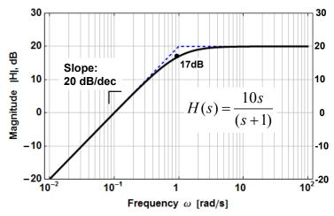
Figure 1-5 – Bode plot for the example of (1.22). The plot begins with an upward slope of 20 dB/decade because of the zero at s=0.
