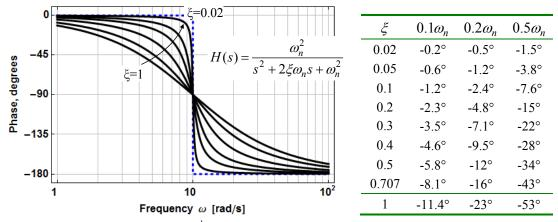
Figure 1-19 – Phase plot for a  $2^{nd}$ -order low-pass response as a function of the damping factor. Numerical data at three frequencies below the break are tabulated as an aid for sketching the response.
