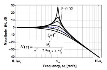
Figure 1-8 – Bode amplitude plot for the general  $2^{nd}$ -order low-pass response for various values of  $\xi$ .
