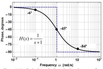
Figure 1-14 – Bode phase plot for a simple pole at s = -1
