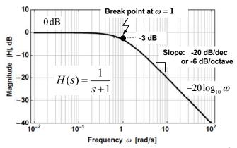
Figure 1-1 – Frequency response for a simple <u>pole</u> at s = -1
