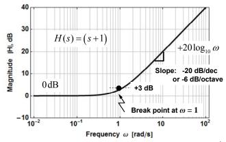
Figure 1-2 – Frequency response for a simple <u>zero</u> at s = -1
