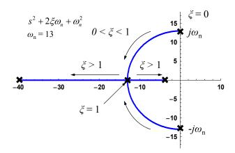
Figure 1-13 – Root-locus in the complex plan for the second-order polynomial as a function of damping factor.
