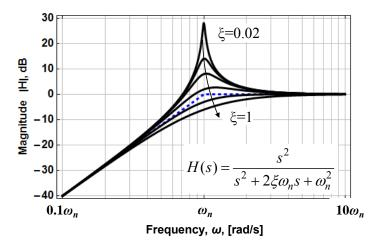
Figure 1-11 – Amplitude response for the general  $2^{nd}$ -order highpass function for various values of  $\xi$ .
