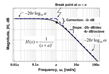
Figure 1-3 – Bode plot for a repeated pole at s = -a. The dashed line is a quick estimate called the "uncorrected" Bode plot. The solid line is the "corrected" Bode plot, passing through the correct location at the break point.
