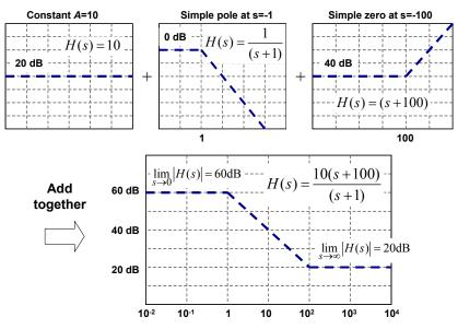
Figure 1-4 – Illustration of how the composite Bode plot of the transfer function in (1.20) is a superposition of the individual terms.
