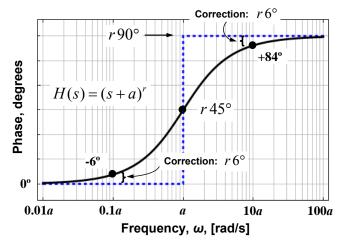
Figure 1-15 – Bode phase plot for a repeated zero at s = -a
