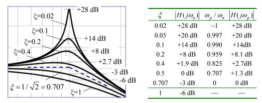
Figure 1-9 – Behavior near the corner frequency for various values of the damping factor  $\xi$ .
