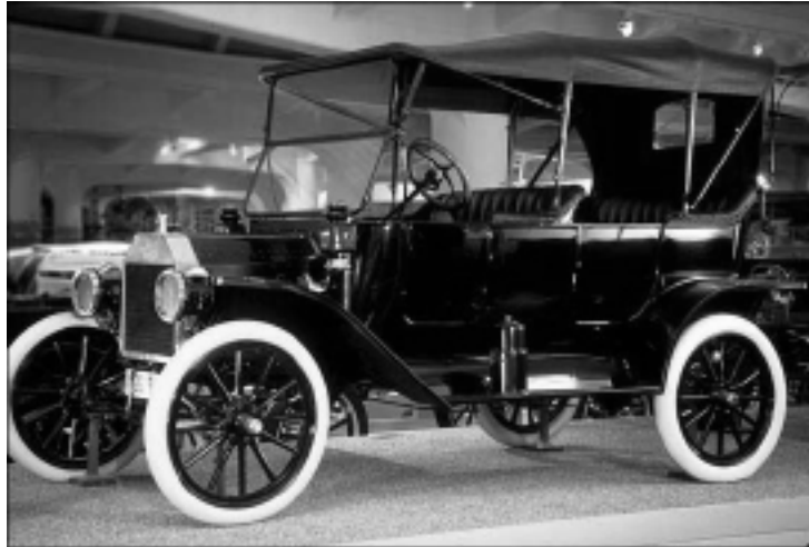
Fig. 1. Ford model-T, the first mass-produced car in history. It was equipped with a cotton band brake, applied to a drum within the gearbox. (Henry Ford Museum)
