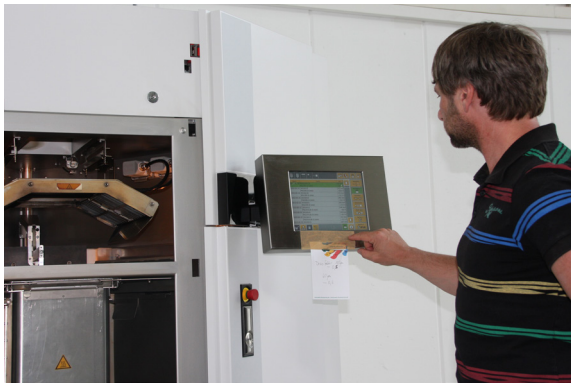
Fast 3-D printing opportunity: Laser sintering with EOS P110 from EOS for high rigidity and quality
